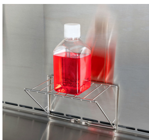
3859000 – Interior Shelf. Stainless steel shelf, 20 x 13 cm (8.0" x 5.0"), mounts to rear grille. Capacity: 1 kg (2.2 lbs.). Shipping weight 0.9 kg (2 lbs.)
