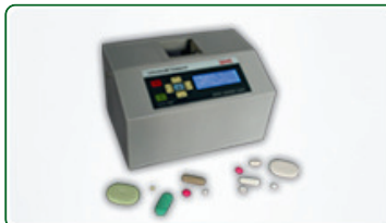
Motorised Tablet Hardness Tester (Model: DHT-150)
