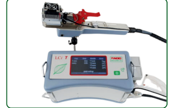
LCI T Compact Photosynthesis System
